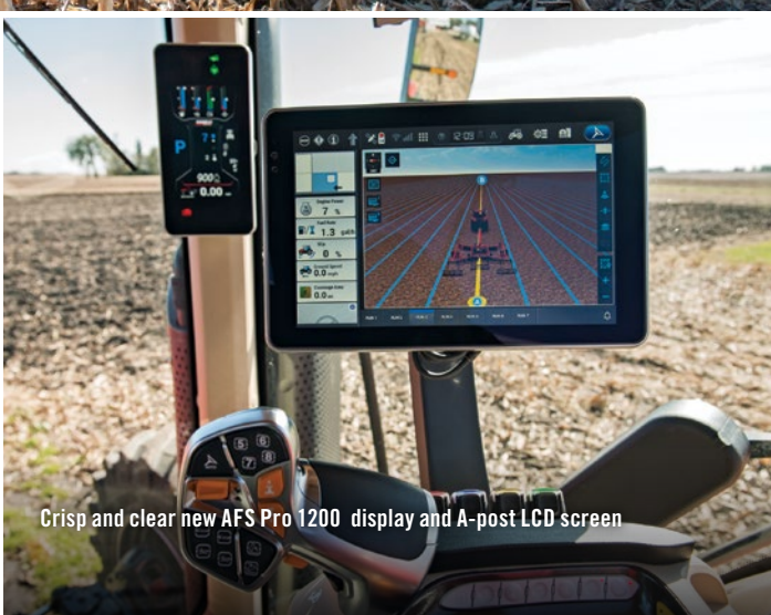
Redesigned Multicontrol armrest and MultiFunction handle
